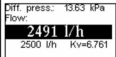
In Kv-mode it is not possible to use the TA-BALANCE procedure, so when trying menu **4 TA BALANCE** you will see:
