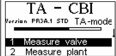
The third line displays the remaining battery capacity (0-100%), here 60%. When the bar is filled to 25% there is a warning message displayed as indicated in the section about **Charging of batteries** (page 7).<sup>4</sup> When this happens, it is important to charge the batteries as soon as possible to avoid unnecessary disruption. Saved measured data are not lost even if the battery capacity is zero. However the instrument cannot be used before charging.
