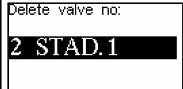
**c)** You may discover that you have made a mistake when making the numbering of the valves. Then you can “move” valves. Example: You have measured on a STAD 25 and given it no 3 and on a STAD 20 that has been given no 5. In reality the STAD 20 should have no 3. Then you can ”move” no 5 to position 3. The STAD 25 will be renumbered to 4 and the old no 4 be a new no 5.....
